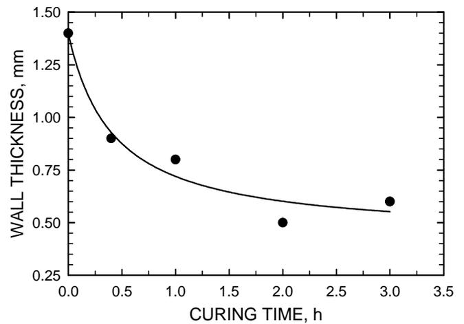
Figure 11. Effect of curing time on the minimum wall thickness required to drill 3.18 mm diameter holes in the gear teeth for part density of 6.8 g/cm<sup>3</sup> (Feed rate: 0.2 mm/rev, Speed: 3420 rpm).
