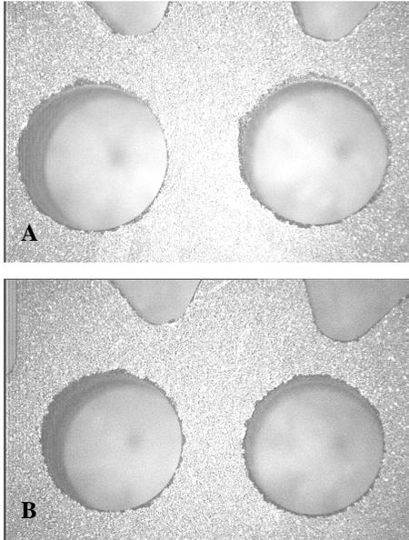
Figure 12. Break-out at the exit of 6.35 mm diameter holes drilled at a feed rate of 0.2 mm/rev and a cutting speed of 3420 rpm cured at 230°C for A) 0.5 h and B) 1.0 h.
