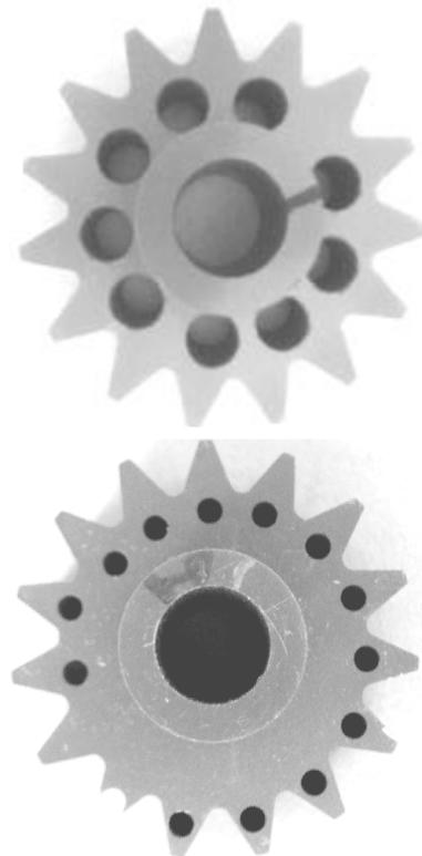
Figure 2. Location of a) 6.34 mm and b) 3.18 mm diameter holes drilled for machinability evaluation.
