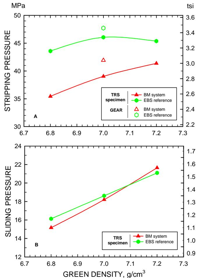
Figure 4. Stripping and sliding pressures required to eject TRS and gears made from BM and EBS lubricating systems.
