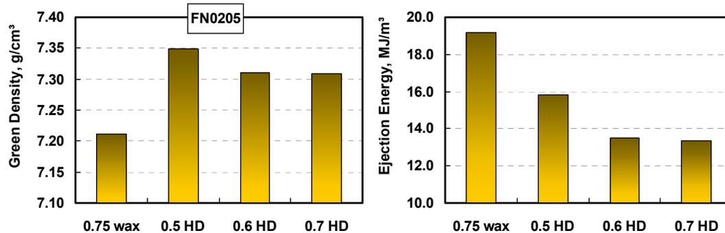
**Figure 10.** Performance of a new lubricant-binder system under development for high density applications. a) Green density b) Ejection energy (FN0205 mixes pressed at 60°C and 840 Mpa)
