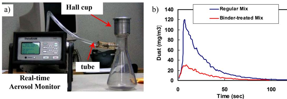
**Figure 3.** Quantity of dust (particles < 10  $\mu\text{m}$ ) created by a regular and a binder-treated F0008 mixes when powders flow in a recipient. a) Experimental assembly b) Results.
