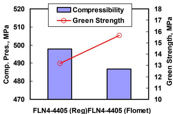
**Figure 8.** Compacting pressure and green strength at 7.0 g/cm<sup>3</sup> for FLN4-4405-1.5% Cu mixes with 0.65% EBS wax. Specimens pressed at 60°C.
