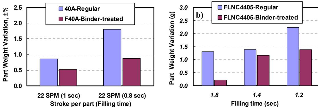
**Figure 5.** Part weight variation for tests carried out under more difficult filling conditions (fill height/wall thickness = 8.2). a) Suction fill b) Gravity fill
