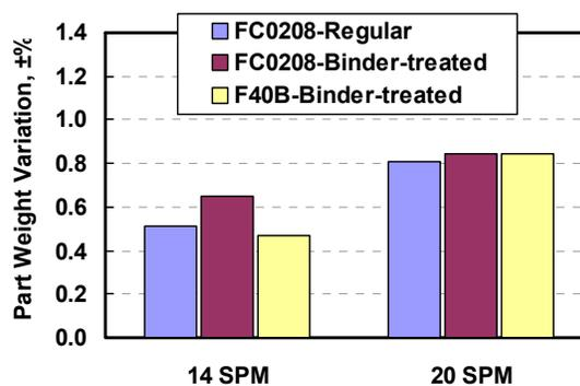
**Figure 4.** Part weight variation for test #1 carried out under easy filling conditions and suction fill (fill height/wall thickness = 2).
