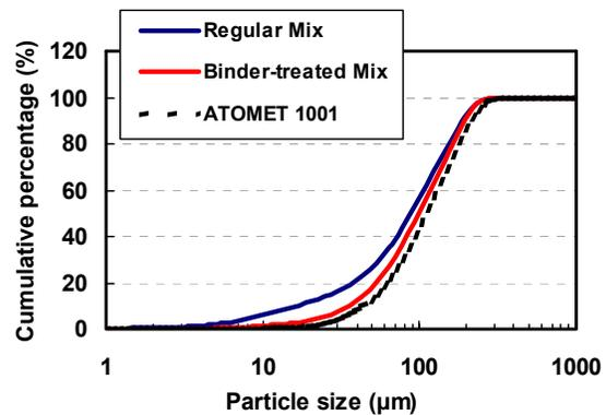
**Figure 2.** Particle size distribution of regular and binder-treated FLOMET mixes (laser diffractometer).
