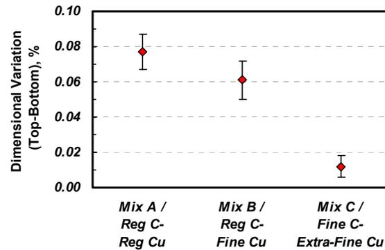
**Figure 7.** Dimensional variation between the top and the bottom of rings made of FLN4-4405 mixes with 4%Ni, 2.6%Cu and 0.5%C.
