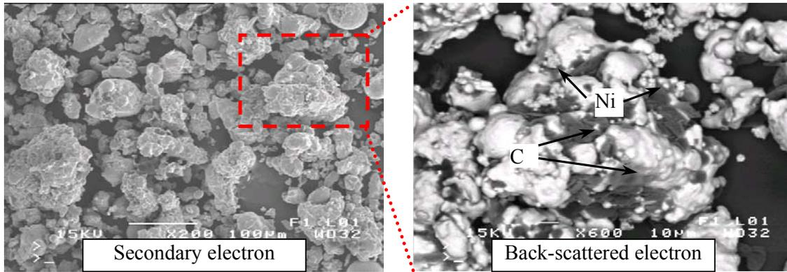
**Figure 1.** SEM micrographs of particles from a binder-treated mix made of ATOMET 1001, 2% Ni, 0.85% graphite and 0.75% wax+binder. C represents either graphite or lubricant.
