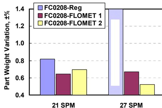
**Figure 6.** Part weight variation obtained during production of drive nuts at two compaction rates. \* Regular mix was not run at 27 SPM.
