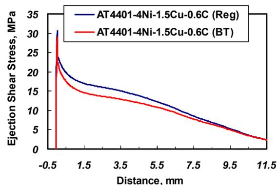
**Figure 9.** Ejection curves for FLN4-4405-1.5% Cu mixes with 0.65% EBS wax. AT4401 refers to ATOMET 4401 (0.85%Mo steel powder).
