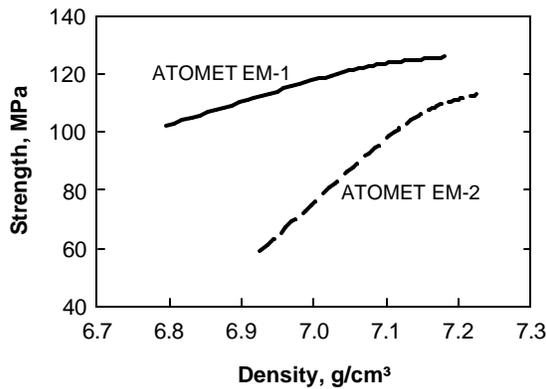
Figure 1. Effect of density on the mechanical strength of TR bars pressed from two SMC
