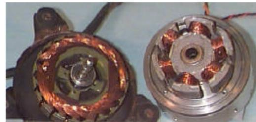
Figure 7. Conventional brush DC motor with a lap winding and the SMC stator of a brushless DC motor with a concentrated winding.
