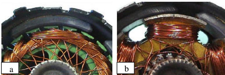
Figure 6. Armature of a brush DC motor: a) laminated structure with lap winding; b) SMC structure with concentrated windings.
