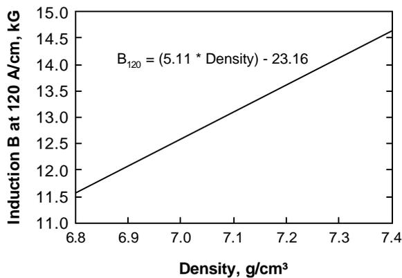
Figure 2. Effect of density of SMC materials on the magnetic induction at an applied field of 120 A/cm.
