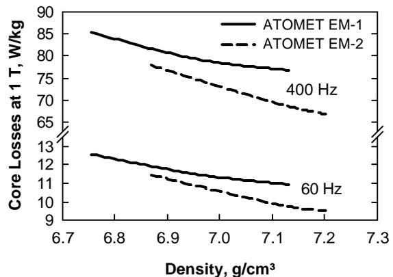
Figure 3. Effect of density on the total core losses at 1 Tesla measured at 60 and 400 Hz.
