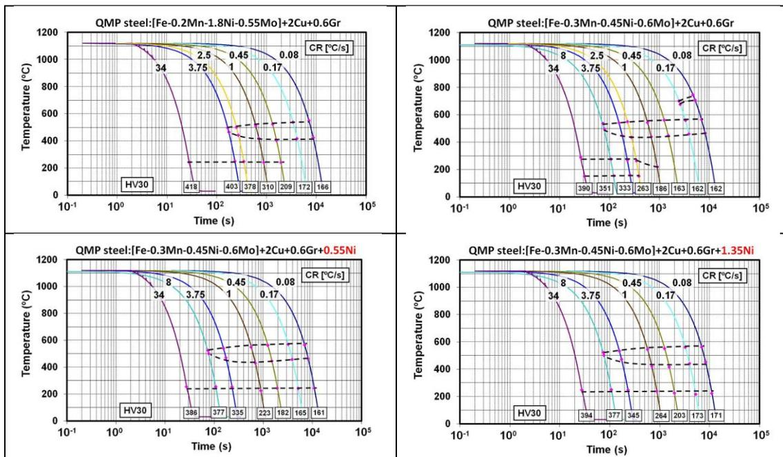
Figure 1.- CCT curves for (a) fully pre-alloyed 4601 steel grade, and for 4201-based steels with various elemental Ni additions: (b) 0% Ni, (c) 0.55%Ni and (d) 1.35%Ni. In all cases graphite and copper additions were kept constant at 0.6 and 2%wt respectively.
