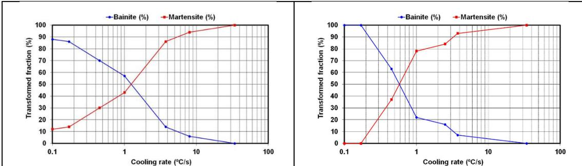
Figure 2.- Phase quantification as a function of cooling rate for (a) 4201+1.35%Ni+2%Cu, and (b) fully pre-alloyed 4601+ 2%Cu steel grades.
