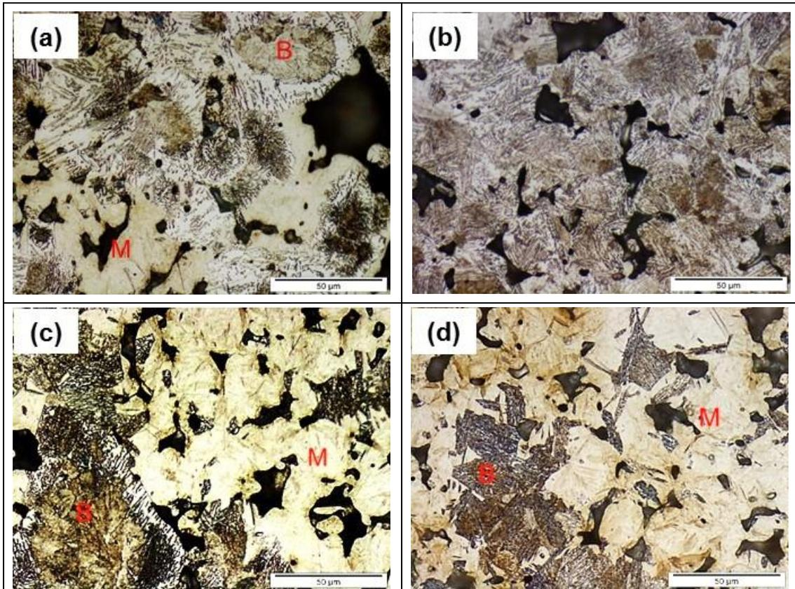
Figure 3.- Microstructures after  $1120^{\circ}\text{C}$ , 15 min for 4201+1.35%Ni (left column) and 4601 (right column). Cooling rates (a, b)  $0.17^{\circ}\text{C/s}$  above and (c, d)  $1.0^{\circ}\text{C/s}$ .
