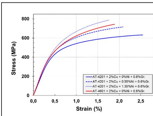
Figure 6.- Tensile curves for the indicated powder mixtures.
