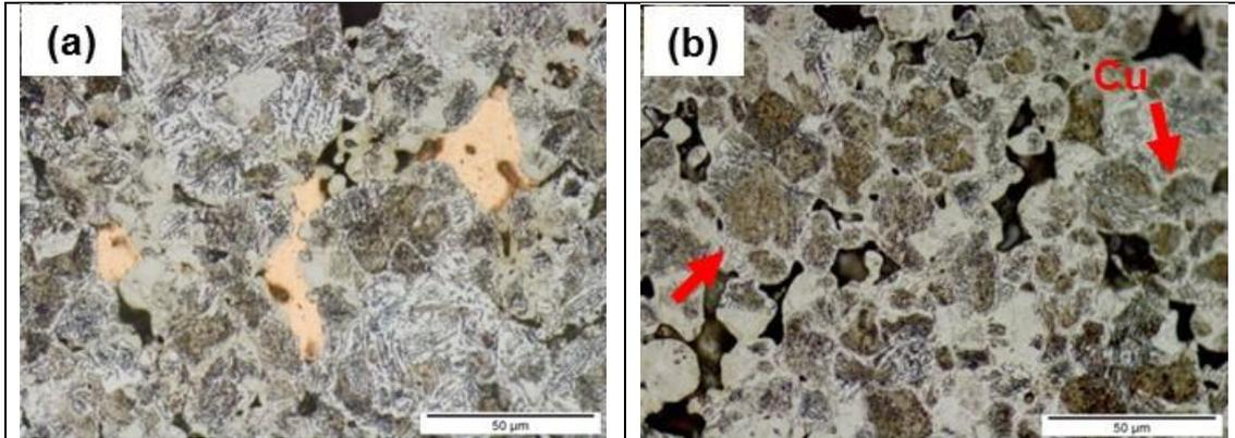
Figure 4.- Microstructural evolution for AT4601+2Cu as revealed by interrupted sintering experiments at (a) 1076 and (b) 1090°C followed by cooling at  $\sim 0.17^\circ\text{C/s}$ .
