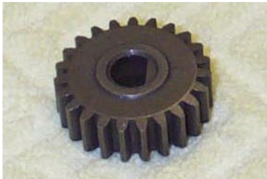
Figure 3. A gear manufactured with FLOMET 44A
