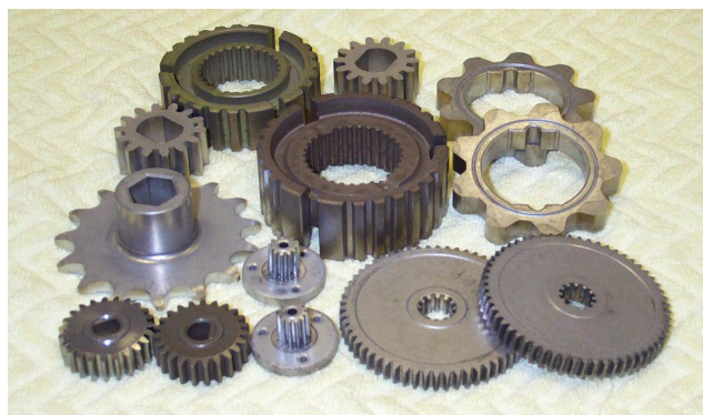
Figure 2. Parts manufactured with FLOMET 44A & 44B
