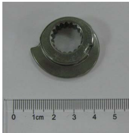
Figure 7. Picture of the eccentric inner gear used for the HD lubricants Test.
