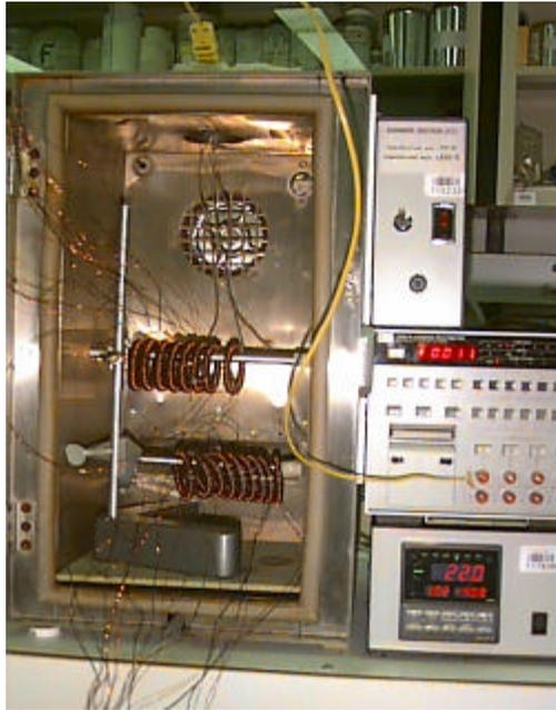
Figure 1: Thermal chamber assembly with the temperature programmer and recorder.
