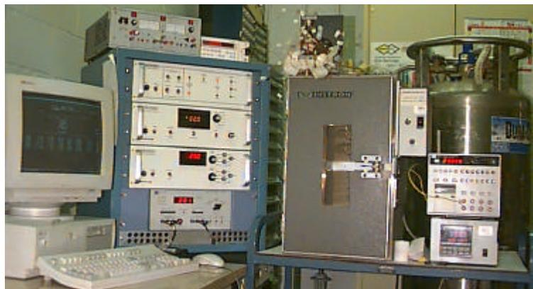
Figure 2: Complete assembly with the thermal chamber and magnetic characterization system.
