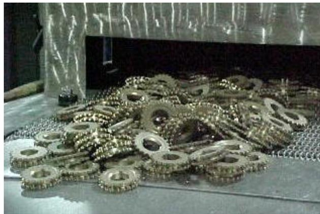
Figure 6. Green machined sprockets in production.
