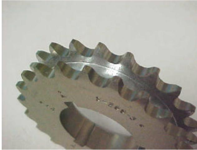
Figure 4. Surface finish of green machined parts at tuning speed of 900 rpm and feed rate 0.2mm/rev.
