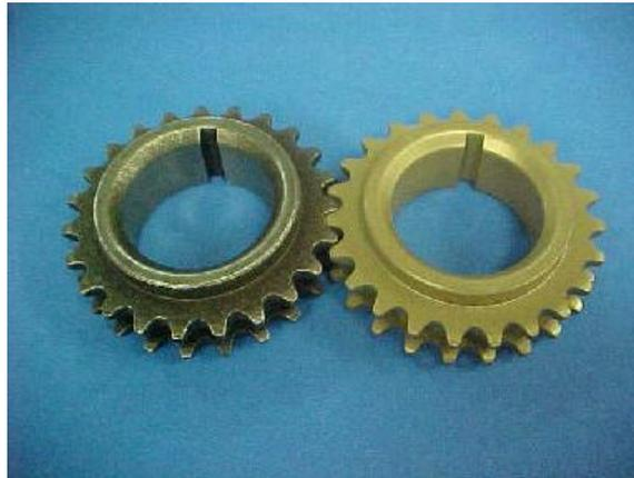
Figure 1. Typical Timing Sprocket.
