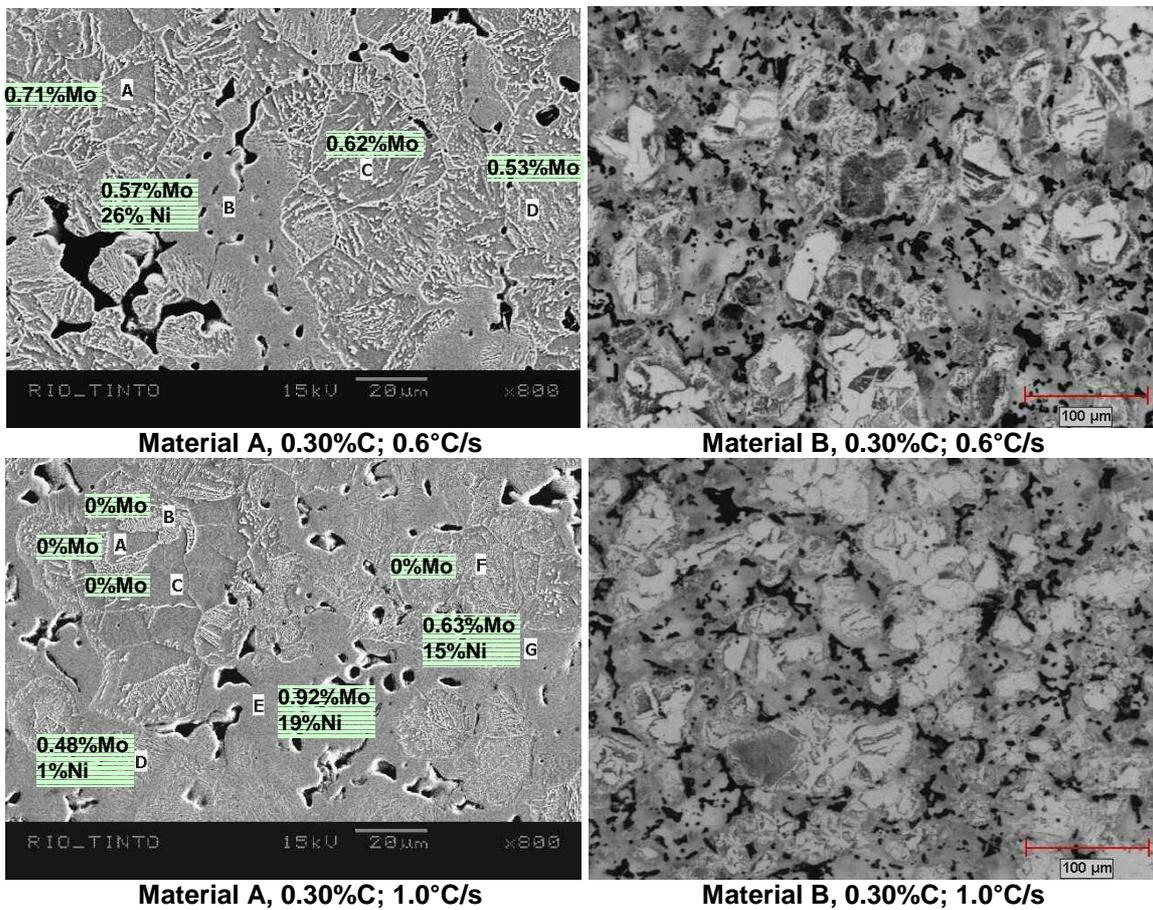
Figure 3. Microstructure of materials A and B containing 0.30% C and cooled at 0.6 and 1.0°C/s (Nital etched, 200X).
