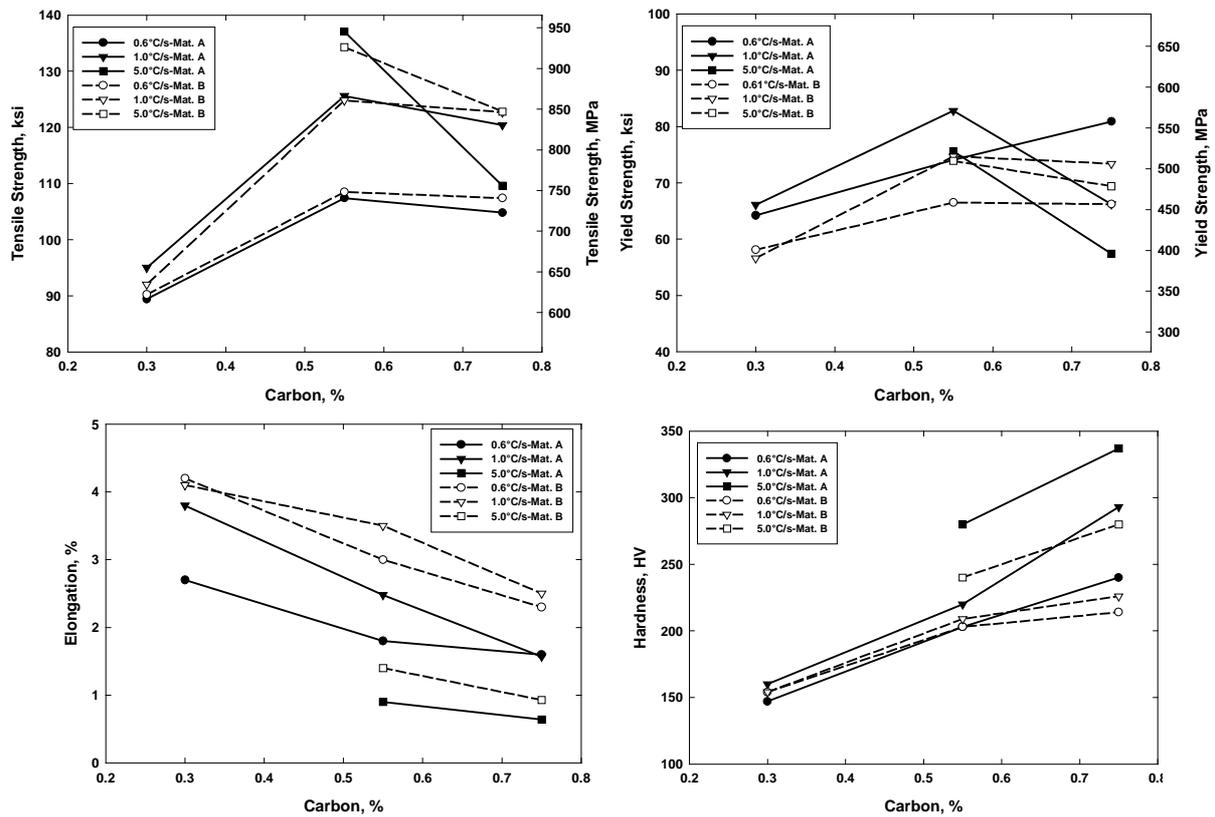
Figure 2. Effect of carbon concentration and cooling rate on tensile properties and apparent hardness of specimens pressed to 7.0 g/cm³ from powder A and B.
