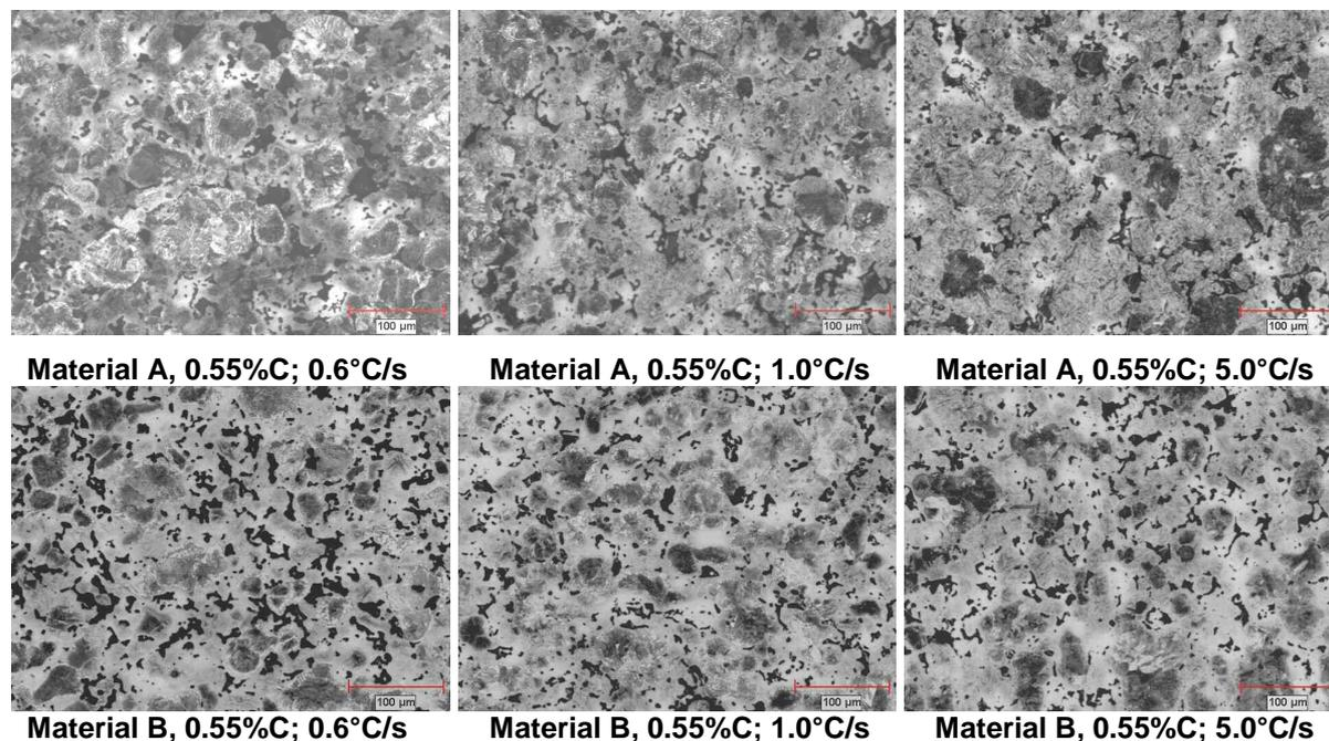
**Figure 4. Microstructure of materials A and B containing 0.55%C and cooled at 0.6 and 1.0 and 5.0°C/s (Nital etched, 200X).**
