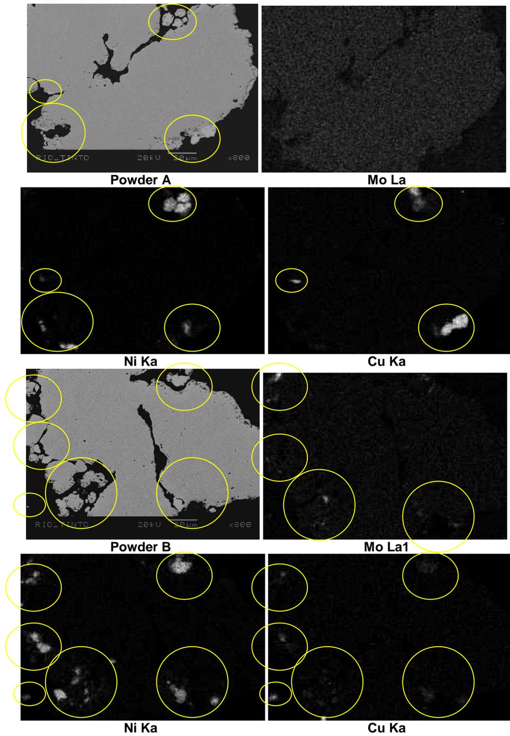
**Figure 1. Distribution of Mo, Ni and Cu in powder A and B.**
