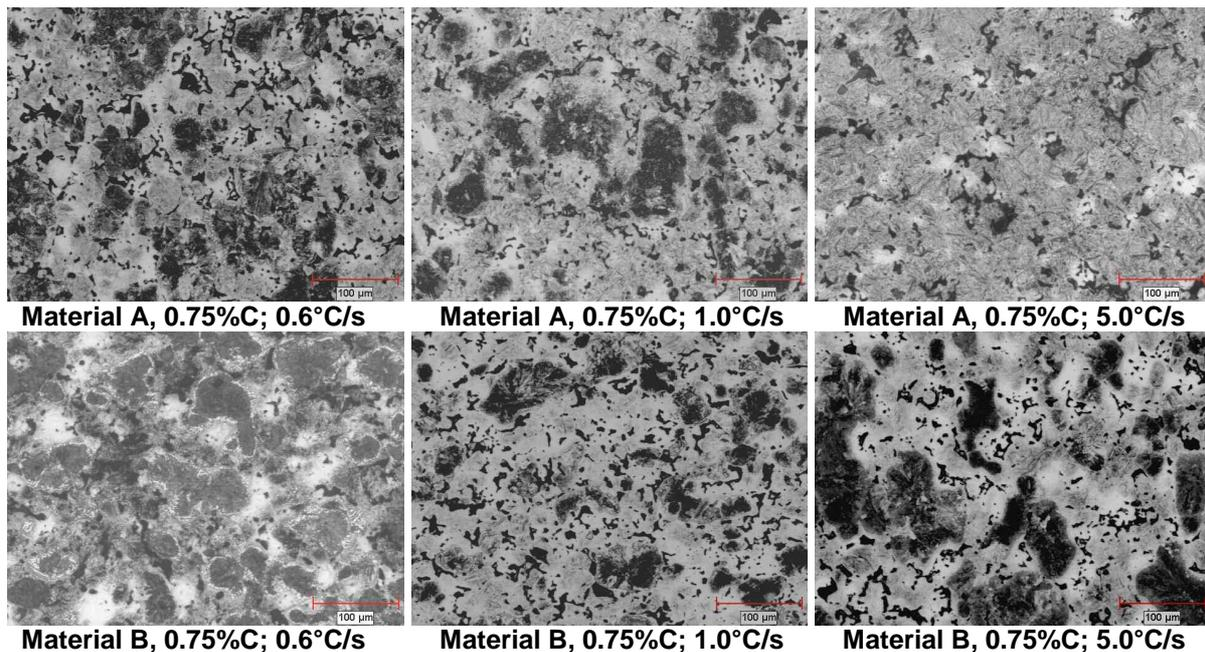
**Figure 5. Microstructure of materials A and B containing 0.75%C and cooled at 0.6 and 1.0 and 5.0°C/s (Nital etched, 200X).**
