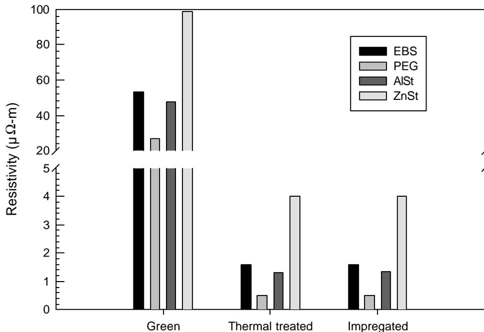
**Figure 4.** Effect of a thermal-treatment at 500°C for 30 minutes in N<sub>2</sub> and resin-impregnation on the electrical resistivity of specimens pressed at 620 MPa/65°C from mixes containing 0.75 % of different lubricants.
