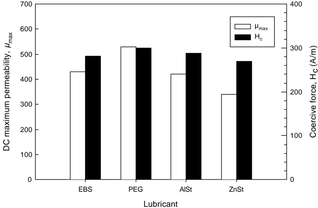
**Figure 7.** DC maximum permeability and coercive force  $H_c$  ( $B = 11.9$  kA/m or 150 Oe) of specimens pressed at 620 MPa/65°C, heated 30 min at 500°C in  $N_2$  and resin-impregnated.
