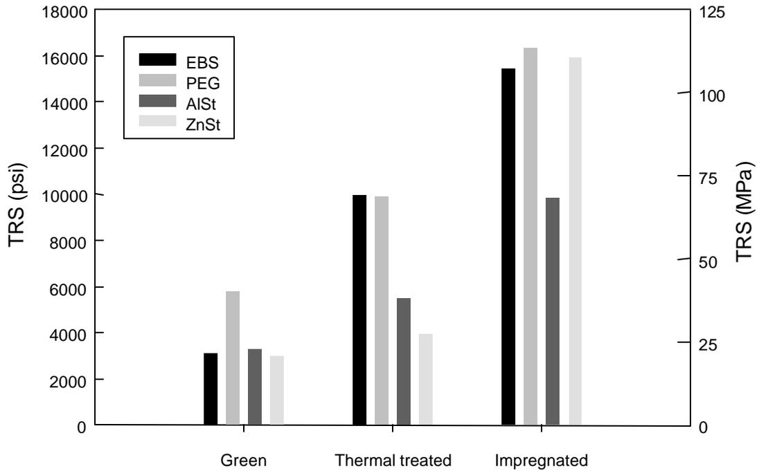
**Figure 5.** Transverse rupture strength of specimens compacted at 620 MPa/65°C using iron-0.75 % lubricant mixes.
