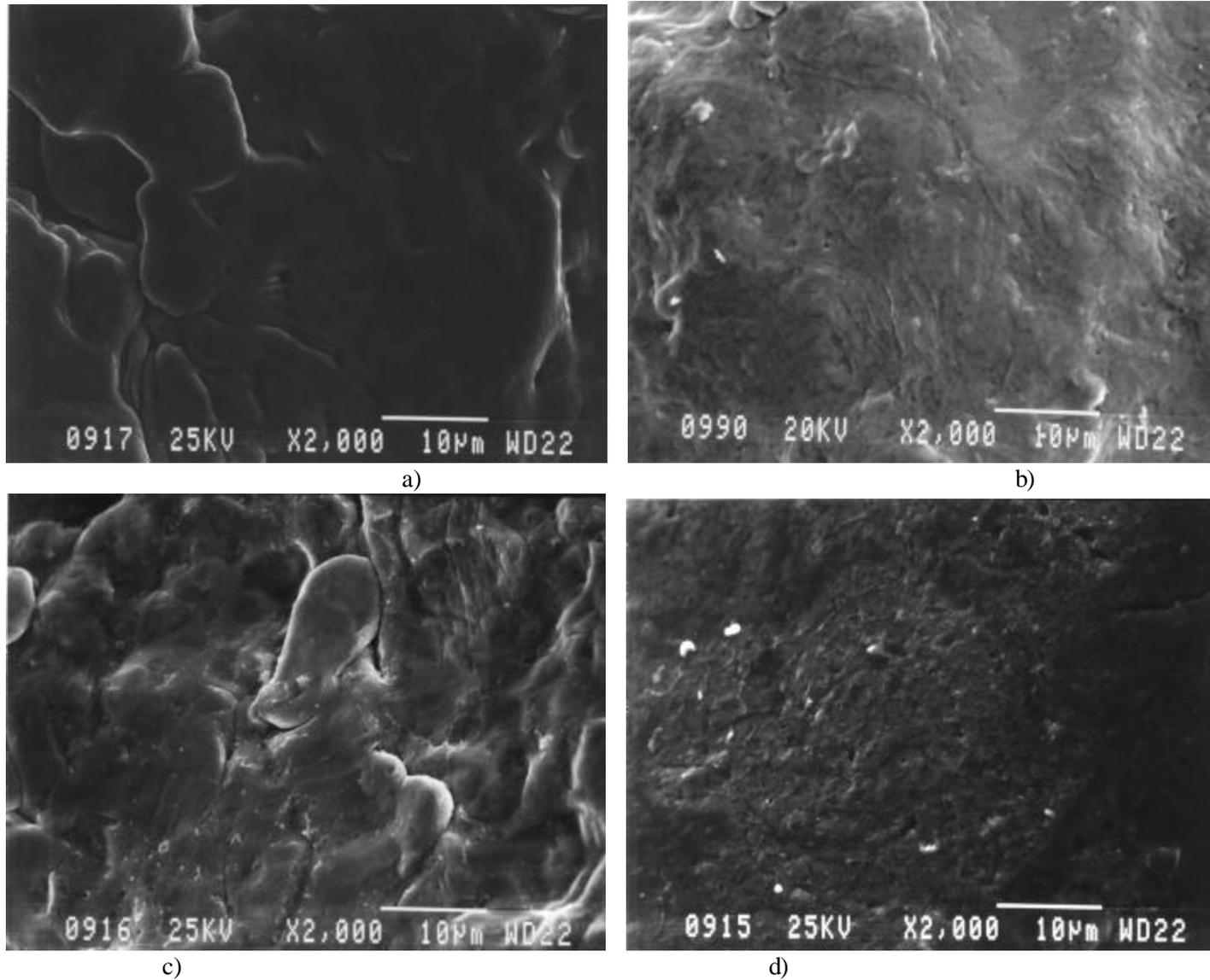
**Figure 3.** Fracture surface of TRS bars fabricated with different lubricants (pressed at 620 MPa/65°C and heated 30 minutes at 500°C in N<sub>2</sub>): a) EBS b) PEG c) Zn-St d) Al-St.
