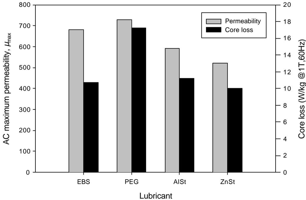
**Figure 8.** AC permeability (60 Hz) and core losses (1 T/60 Hz) of specimens pressed at 620 MPa/65°C, heated 30 min at 500°C in N<sub>2</sub> and resin-impregnated.
