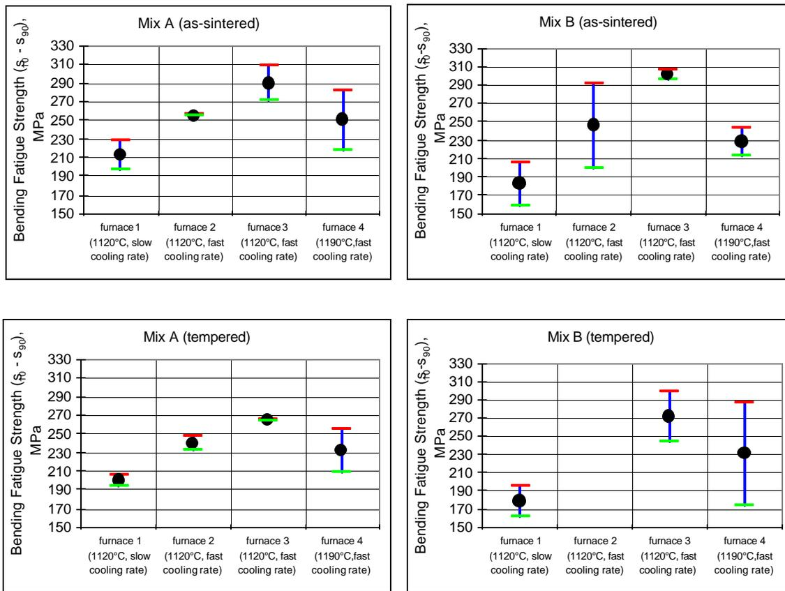
**Figure 2:** Bending fatigue strength of material A and material B
