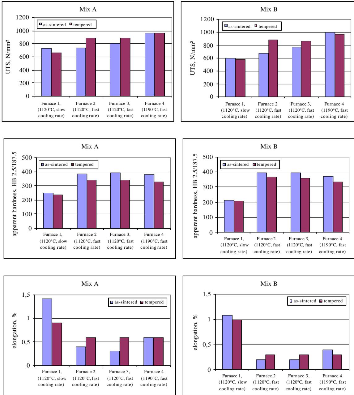
**Figure 1:** Effect of sintering conditions on tensile strength, apparent hardness and elongation of as-sintered and tempered (200°C/60 min/air) specimen
