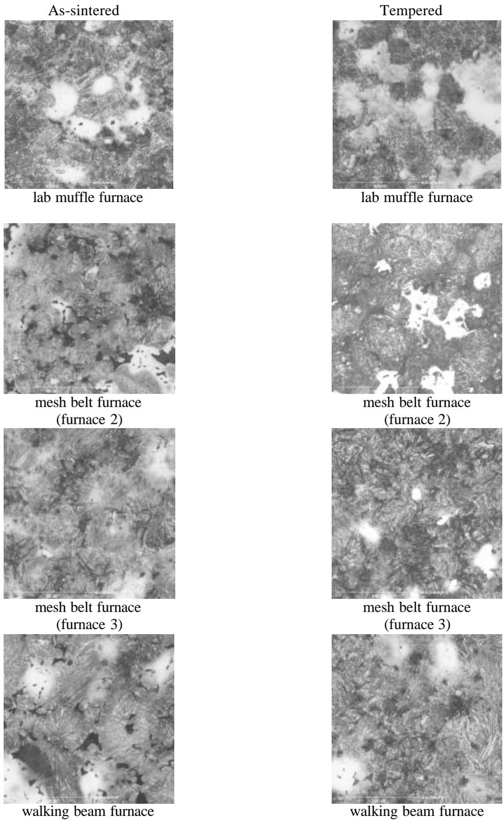
**Figure 5:** Micrographs of test bars made from material B, sinter conditions see Table 2 (ATOMET DB49L + 0,50% graphite + 0,75% wax)
