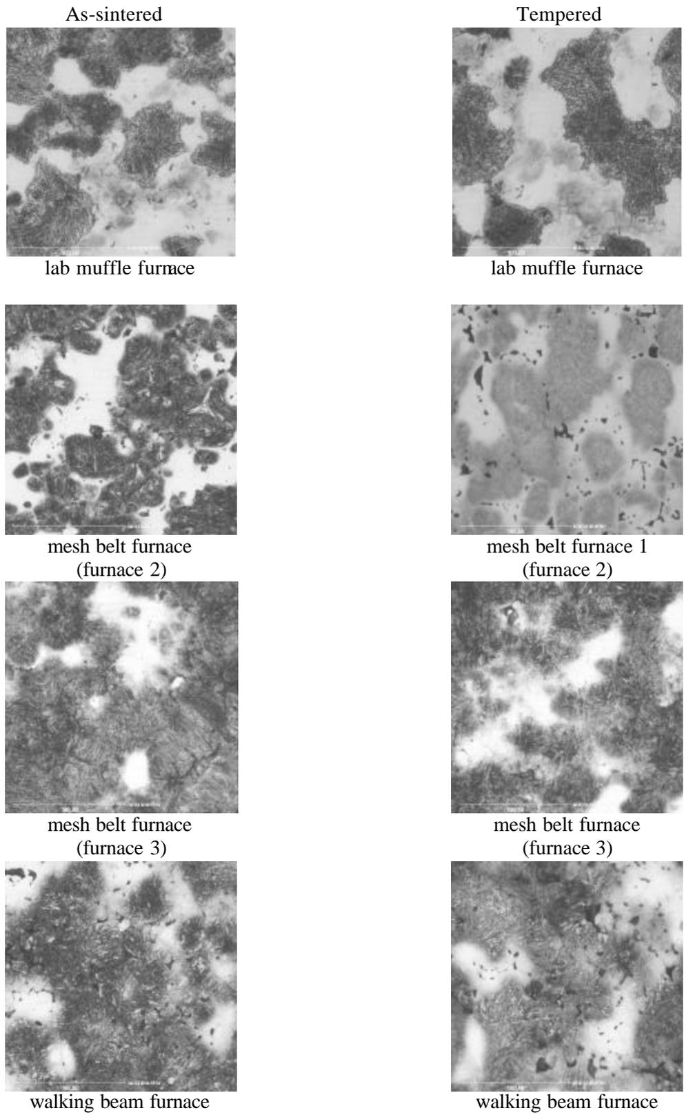
**Figure 4:** Micrographs of test bars made from material A, sinter conditions see Table 2 (ATOMET DB49 + 0,50% graphite + 0,75% wax)
