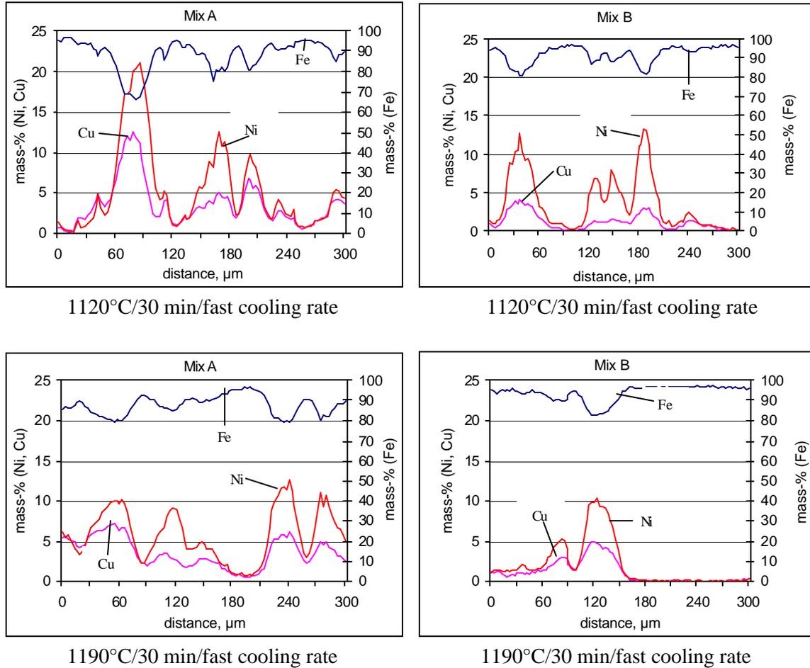
**Figure 3:** line scans of material A and B after sintering and tempering (200°C/60 min/air)
