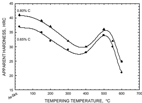
**Figure 14. Effect of tempering temperature on apparent hardness of specimens pressed from powder C with 2% Cu and various amounts of combined carbon [4] ( $7.0\text{g}/\text{cm}^3$ ,  $0.6^\circ\text{C}/\text{s}$  in the range of 650 to 400°C).**
