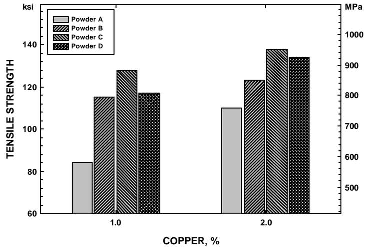
**Figure 8. Effect of copper content on tensile strength of sinter hardened materials (0.5%C cooled at 1.5°C/s and tempered at 200°C).**
