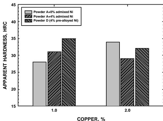
**Figure 9. Effect of admixing Ni on apparent hardness of sinter hardened materials containing either 1 or 2% Cu and 0.7%C (cooled at 1.5°C/s and tempered at 200°C, 6.85 g/cm<sup>3</sup>).**
