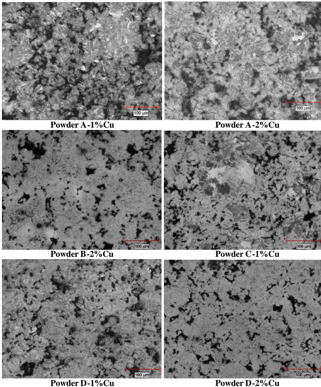
**Figure 7. Microstructure of materials containing 1 or 2% copper and 0.5% combined carbon, sintered at 1135°C and cooled at 1.5°C/s.**
