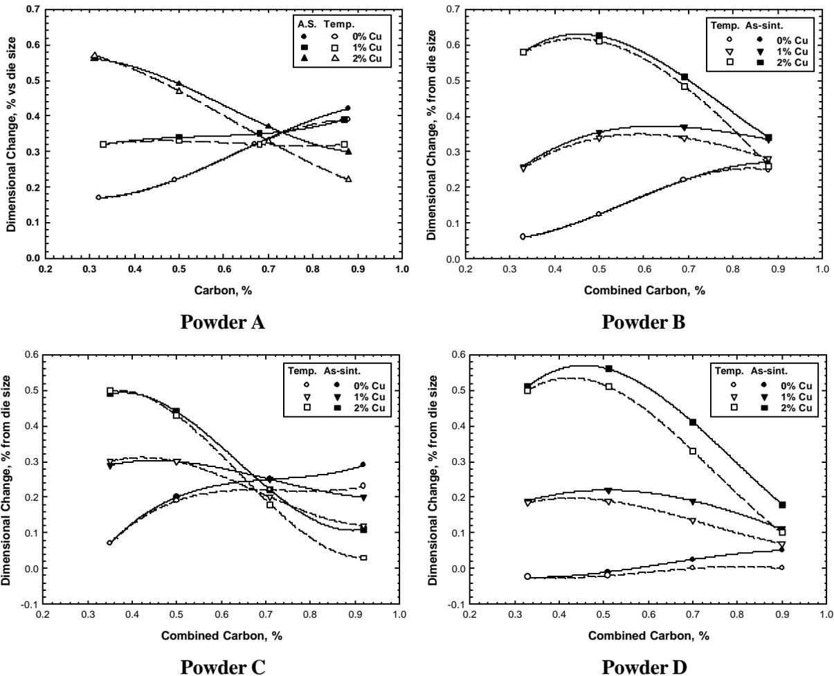
**Figure 16. Effect of carbon and copper concentrations and tempering at 200°C on dimensional change of specimens pressed at 6.9 g/cm<sup>3</sup> with the four powders, sintered at 1135°C and cooled at 1.5°C/s in the range of 650 to 400°C.**
