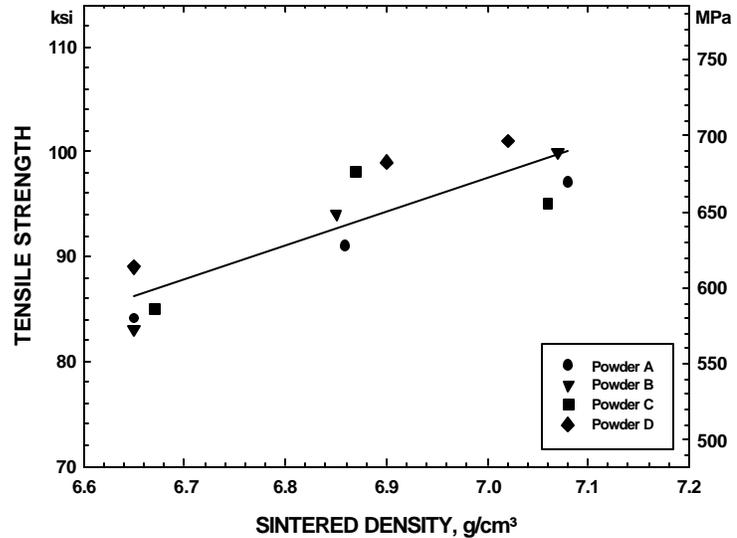
Figure 5. Effect of sintered density on tensile strength of sinter hardened materials (1%Cu/0.9%C cooled at 1.5°C/s and tempered at 200°C).
