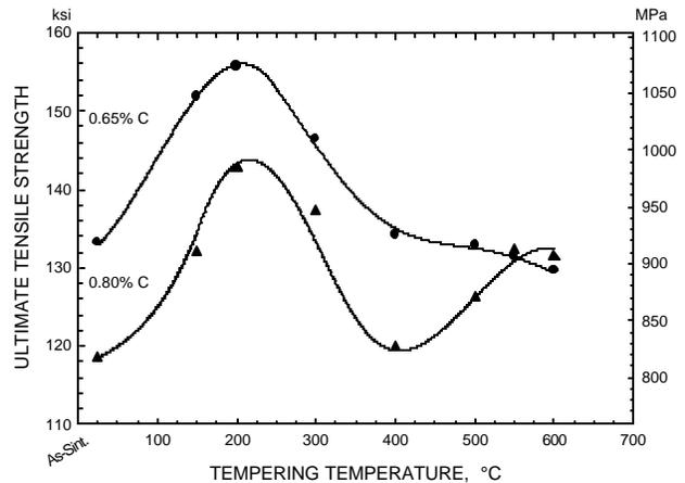
**Figure 15. Effect of tempering temperature on tensile strength of specimens pressed from powder C with 2% Cu and various amounts of combined carbon [4] ( $7.0\text{g}/\text{cm}^3$ ,  $0.6^\circ\text{C}/\text{s}$  in the range of 650 to 400°C).**
