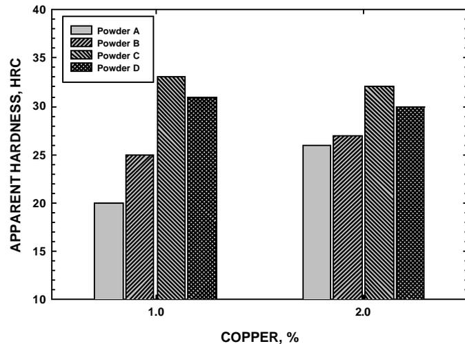
Figure 6. Effect of copper content on apparent hardness of sinter hardened materials (0.5%C cooled at 1.5°C/s and tempered at 200°C).
