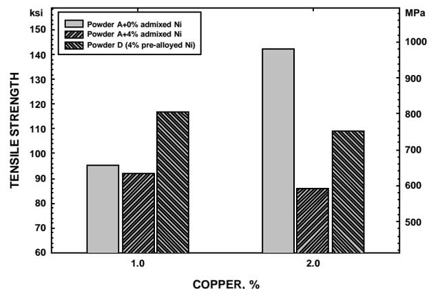
**Figure 10. Effect of admixing Ni on tensile strength of sinter hardened materials containing either 1 or 2% Cu and 0.7%C (cooled at 1.5°C/s and tempered at 200°C, 6.85 g/cm<sup>3</sup>).**
