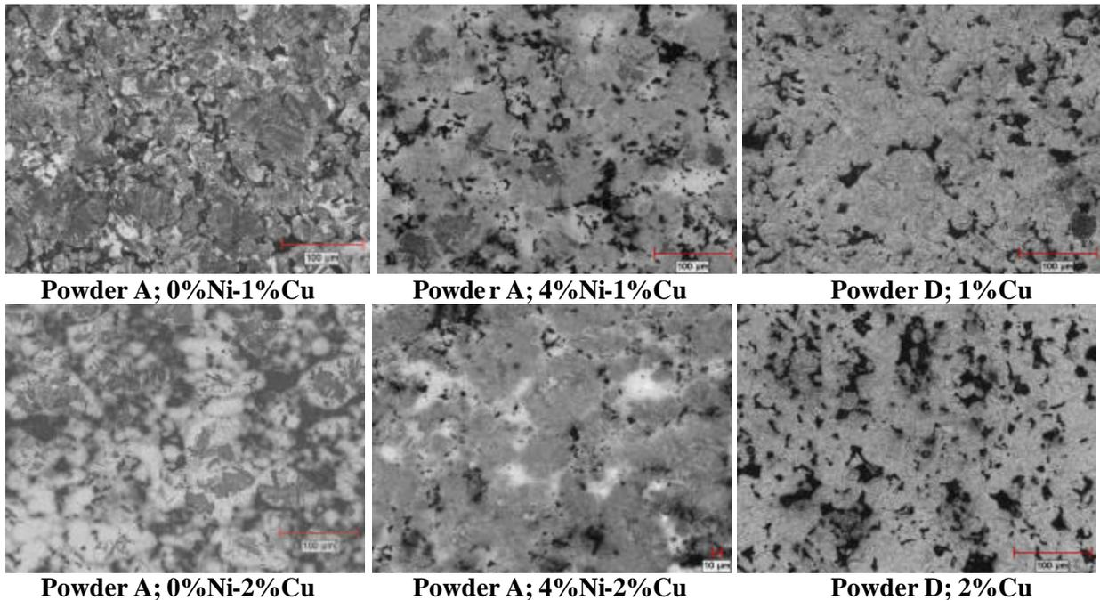
**Figure 11. Microstructure of specimens pressed with powder A and containing either 0 or 4% admixed Ni and from powder D containing 4% pre-alloyed Ni (1 or 2% Cu and 0.7% C, cooled at 1.5°C/s).**
