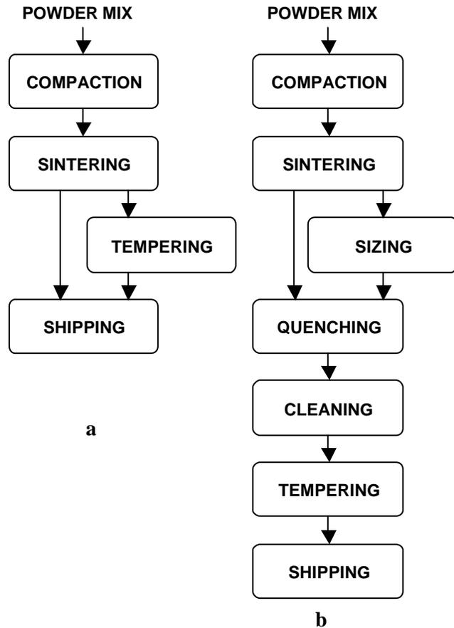
**Figure 1. Comparison of the sinter hardening and quench and temper process.**
