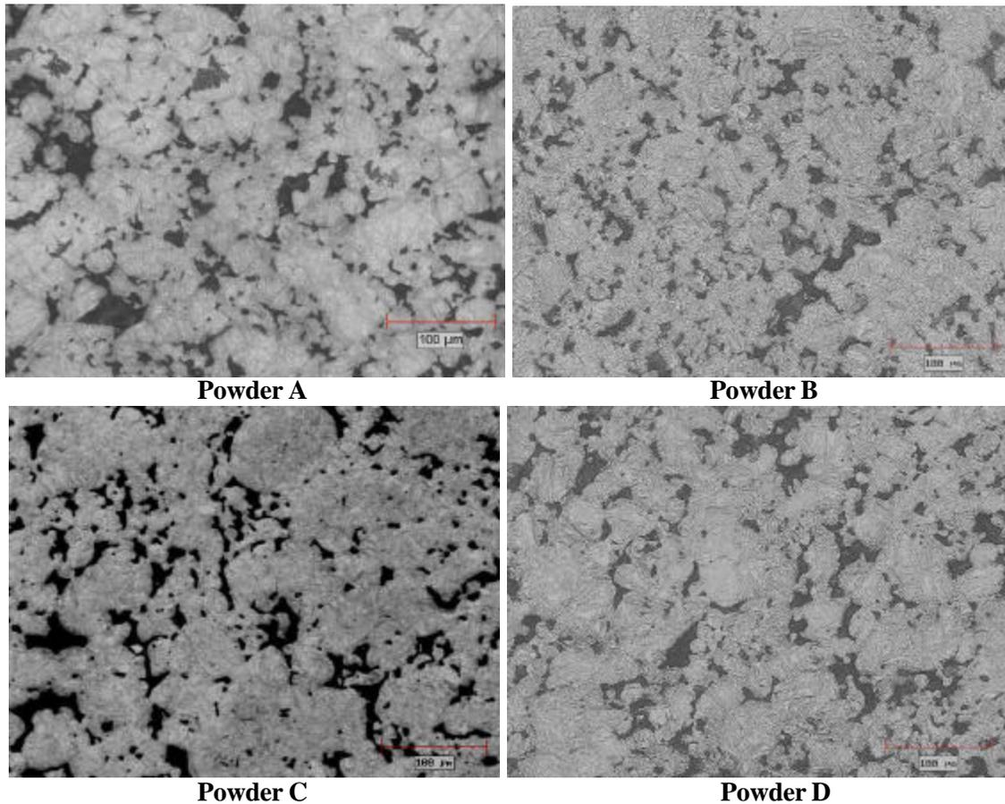
**Figure 4. Microstructure of specimens prepared from the various powders (1%Cu-0.9%C, cooled at 1.5°C/s).**
