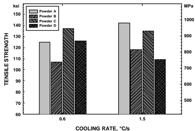
**Figure 13. Effect of cooling rate in the range of 650 to 400°C on ultimate tensile strength of sinter hardened materials (0.7%C-2%Cu; tempered at 200°C).**
