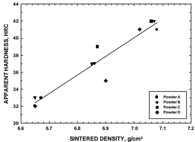
**Figure 3. Effect of sintered density on apparent hardness of sinter hardened materials (1%Cu/0.9%C; cooled at 1.5°C/s and tempered at 200°C).**
