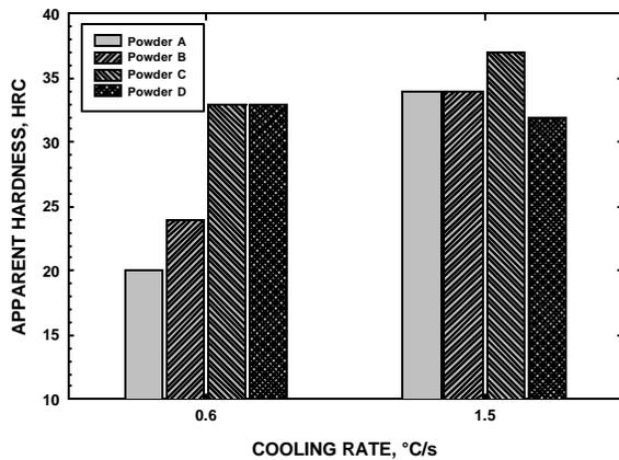
**Figure 12. Effect of cooling rate from 650 to 400°C on apparent hardness of sinter hardened materials (0.70%C-2%Cu; tempered at 200°C).**
