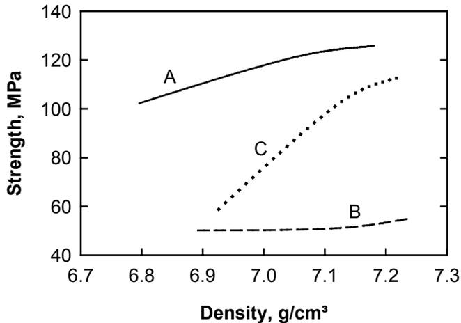
Figure 3. Effect of density on the mechanical strength of TR bars for the three materials cured 30 min in air : material A at 200°C, B at 160°C and C at 350°C.
