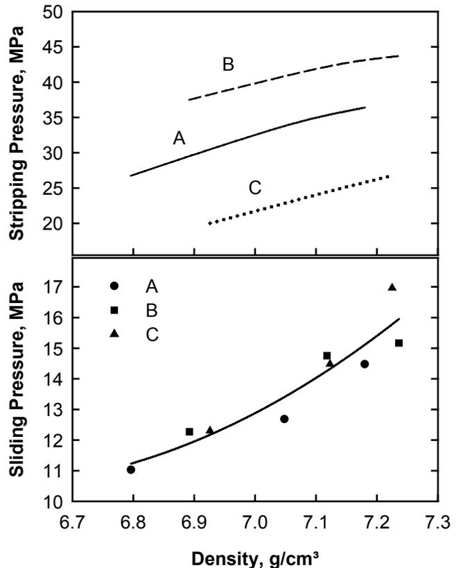
Figure 2. Effect of density on the stripping and sliding ejection pressures of 12.7 mm thick TR bars pressed from the three composite materials.
