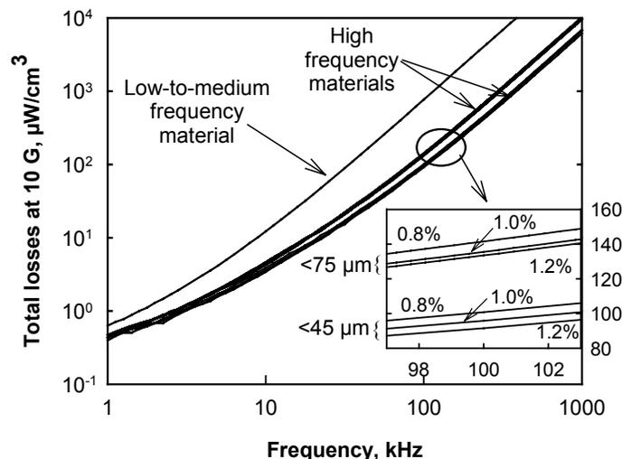
Figure 8. Total losses at 1 mT for high frequency materials compared with a low-to-medium frequency material. The inset at 100 kHz shows the effect of the iron particle size and resin content.
