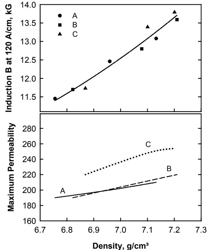
Figure 5. Effect of density on the magnetic induction and maximum permeability (120 A/cm applied field).
