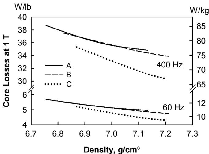
Figure 6. Effect of density on total core losses at 1 Tesla measured at 60 Hz and 400 Hz.
