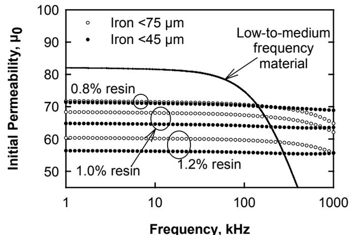
Figure 7. Effect of iron particle size and resin content on the initial permeability at 0.5 mT of high frequency materials and a low-to-medium frequency material.
