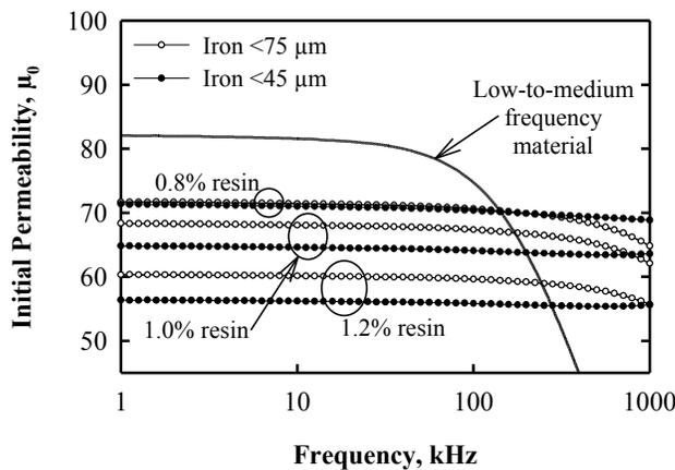
**Figure 4** Effect of iron particle size and resin content on the initial permeability at 0.5 mT of high frequency materials and a low-to-medium frequency material.
