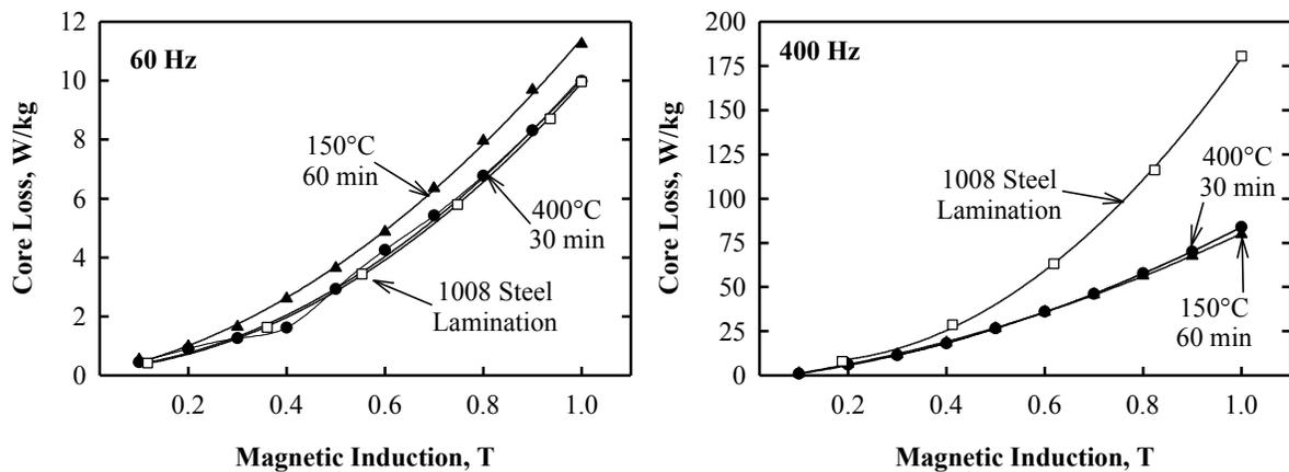
**Figure 3** Core loss comparison at 60 Hz and 400 Hz between a reference low carbon steel (AISI 1008) and iron/0.8% resin composites pressed at 620 MPa/65°C and cured at 150°C and 400°C.
