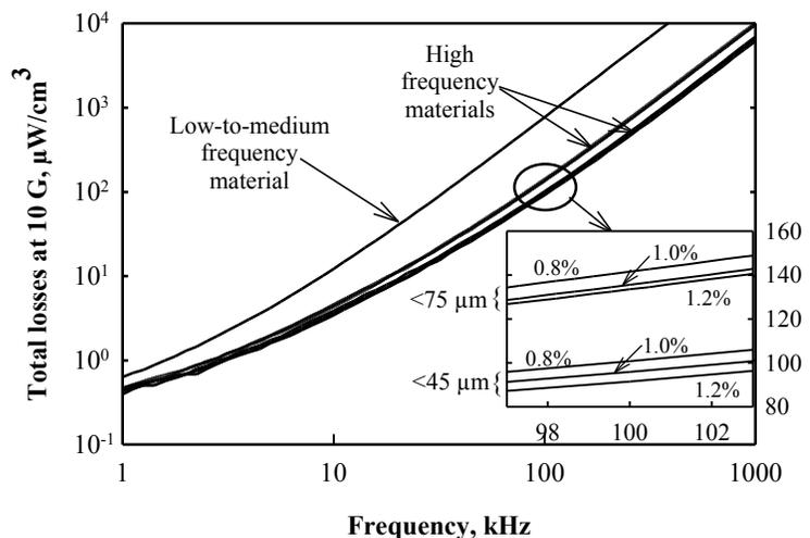
**Figure 5** Total losses at 1 mT of high frequency materials compared with a low-to-medium frequency material. The inset at 100 kHz shows the effect of the iron particle size and resin content.
