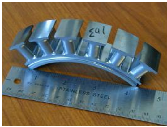
Figure 1 : Stator segment compacted from the press-ready powder mix used in this study.
