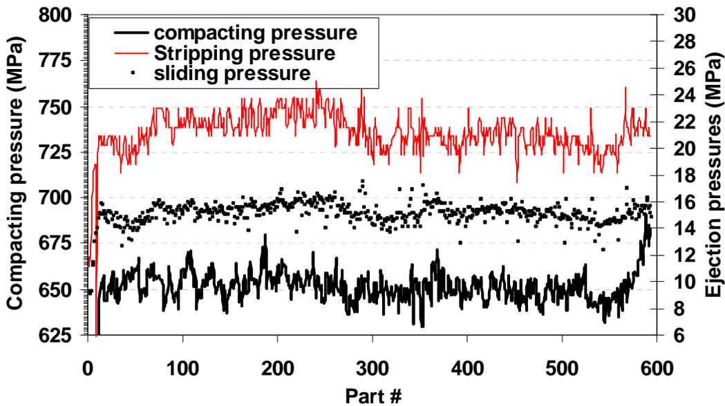
**Figure 11:** Part-to-part compacting pressure and ejection stability of half inch thick Izod bars pressed with Mix 1 at a density of 7.20 g/cm<sup>3</sup>.
