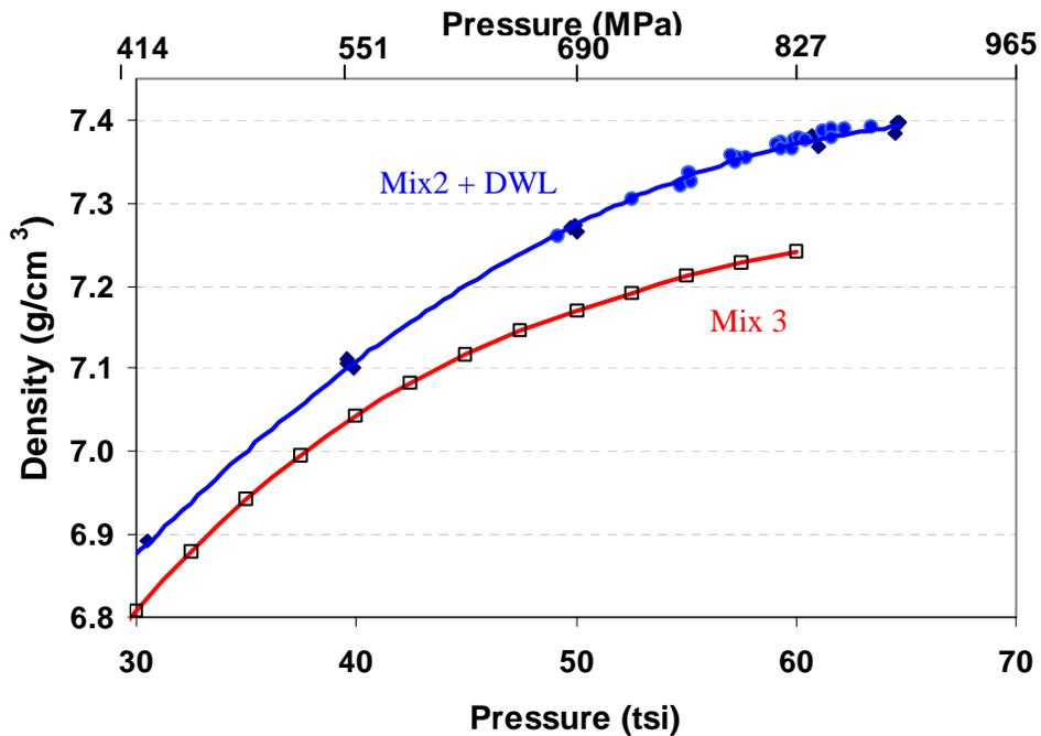
**Figure 8:** Compressibility curve of Mix 2 compacted with DWL as compared to the reference mix, Mix 3
