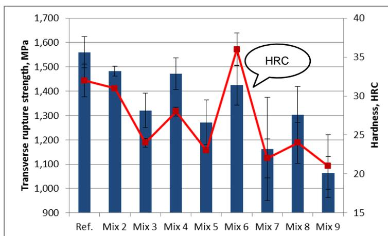
**Fig. 2 Mechanical properties of the mixes containing new additive formulations**
