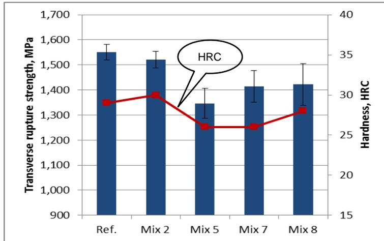
Fig. 4 Transverse rupture strength and hardness of the materials containing experimental additive compared to the reference without additive: sinter-hardened materials
