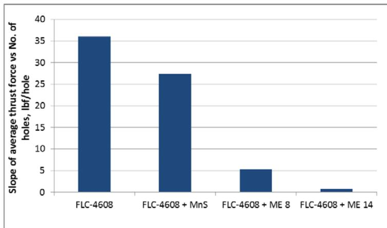
Fig. 11 Slope of average thrust force versus number of holes for different FLC-4608 materials
