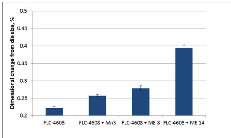
**Fig. 8 Dimensional change from die size of FLC-4608 materials with different machining enhancers**
