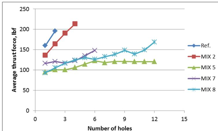
Fig. 5 Drilling machinability of the materials containing select additive formulations compared to the reference without additive: sinter hardened materials
