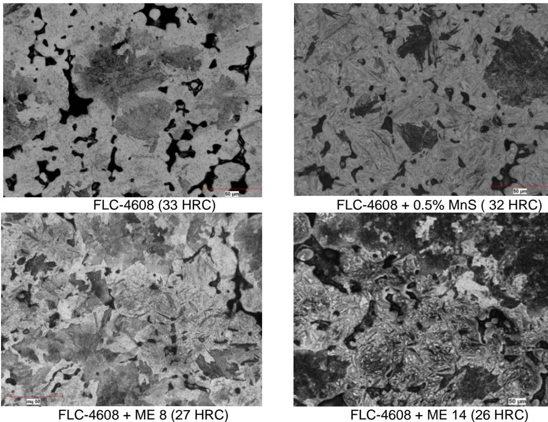
**Fig. 12 Microstructure of different sinter-hardened FLC-4608 materials: center of ½” TRS bars; hardness values in parentheses**
