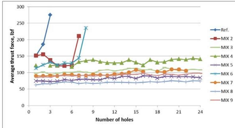
Fig. 3 Drilling machinability of the mixes containing new additive formulations compared to the reference without additive: materials with slow cooling
