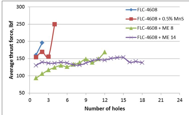
Fig. 10 Drilling machinability in terms of average thrust force of FLC-4608 materials with different machining enhancers
