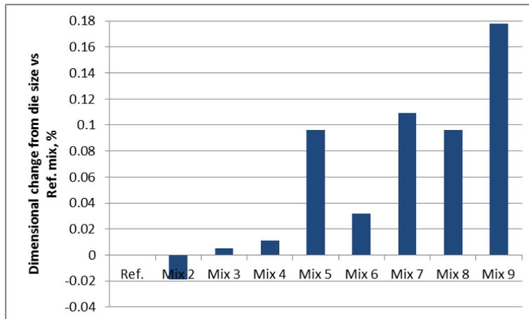
**Fig. 1 Dimensional change from die size: difference with the reference material without machining enhancer**
