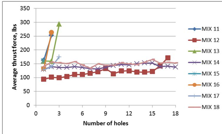
Fig. 6 Drilling machinability of the materials containing the second series of experimental additives
