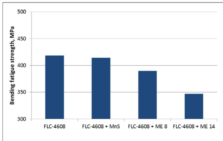
**Fig. 9 Bending fatigue strength of FLC-4608 materials with different machining enhancers: maximum stress at 50% survival rate, loading ratio of 0.1**
