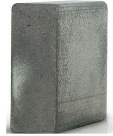
Figure 2. Surface appearance of a green bar with a typical lubricant smear.
