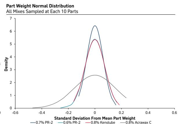
**Figure 3.** Normal distribution of weight calculated from the sampled parts.
