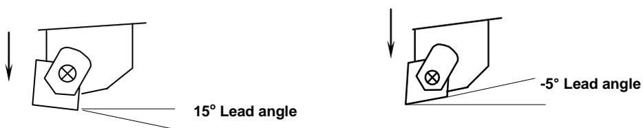
Fig. 1. Tool holder geometry
