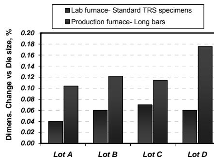
**Figure 6.** Dimensional change measured in lab and production-scale conditions (AT4701).
