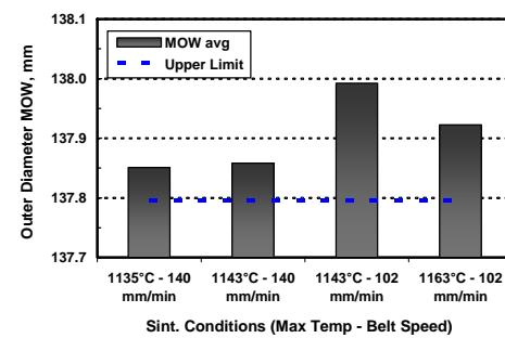
**Figure 7.** Effect of sintering conditions on size for sprockets produced with AT4701.
