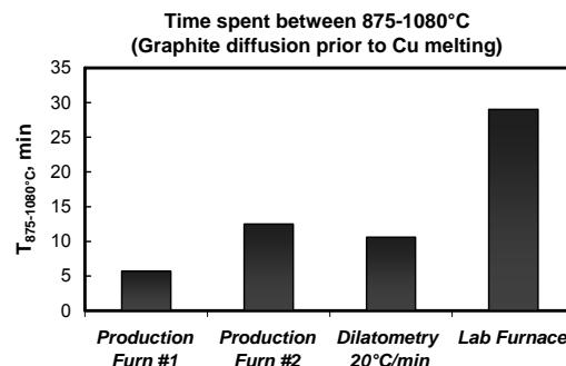
**Figure 9.** Time between 875 and 1080°C for different sintering furnaces.
