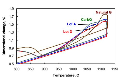
**Figure 8.** Dilatometry curves for Lot A and D
