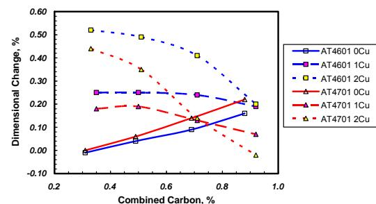
**Figure 1.** Dimensional change as a function of carbon and copper content.
