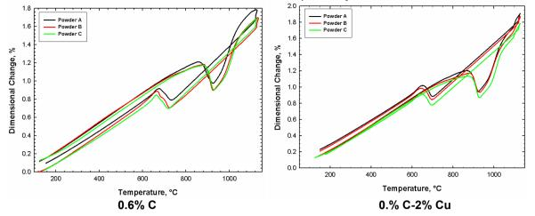
Figure 3. Dilatometry profiles of material A, B and C with 0.6% C and 0.6% C and 2% Cu.
