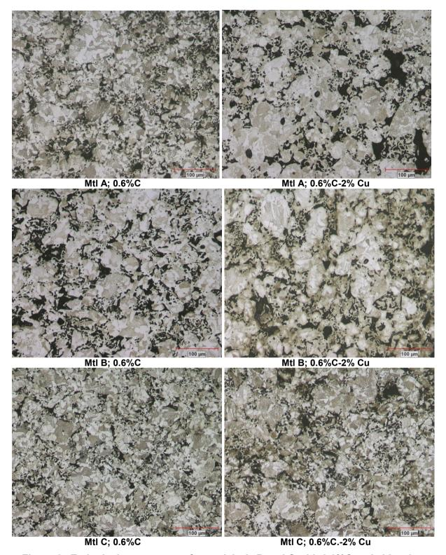
Figure 6. Etched microstructure of materials A, B and C with 0.6%C and either 0 or 2%Cu (natal etched; 200X).
