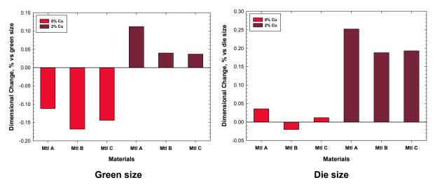
Figure 4. Dimensional change from green and die size of materials A, B and C with 0.6%C and either 0 or 2%Cu (green density of 6.4 g/cm³).
