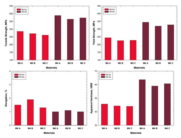
Figure 5. Tensile and yield strengths, elongation and apparent hardness of materials A, B and C with 0.6%C and either 0 or 2.0%Cu (green density of 6.4 g/cm³).
