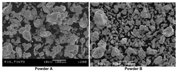
Figure 2. Particle morphology of Powder A and Powder B.
