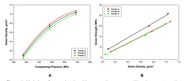
Figure 1. Variation of green density with compacting pressure (A) and green strength with green density (B) of specimens pressed with the three powder grades (mixes containing 0.75% EBS wax).
